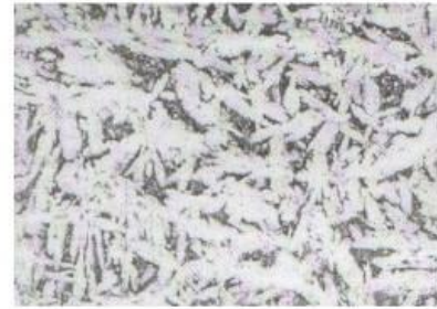
FIGURE 4. MICROSTRUCTURE OF ALLOY, HOT DEFORMED (x960)
